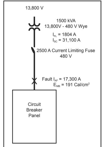
Figure 1: Arc Fault
